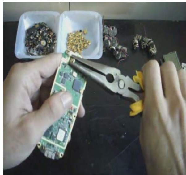
Figure-4. Dismantling of mobile phone PWB (video by Gold-N-Scrap [35]).
