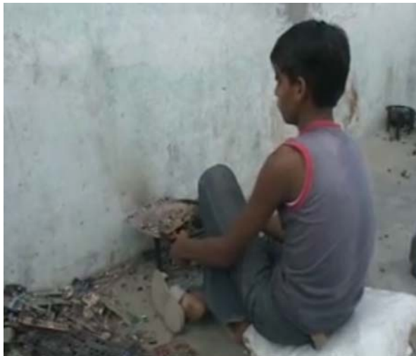
Figure-5. Dismantling of PCB by heating and then hammering by a steel rod (video by Green Peace [30]).
