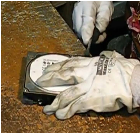
Figure-2. Dismantling of Hard disk - chiseling out the outer lid with chisel (video by e-waste guide [33]).
