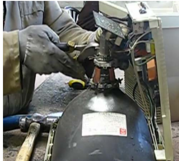
Figure-3. Dismantling of CRT monitor (video by e-waste guide [34]).
