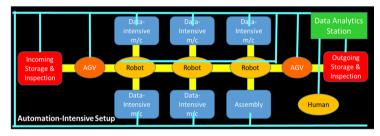
An **Automation-Intensive platform** for high-value manufacturing to showcase what networked automation can offer.
